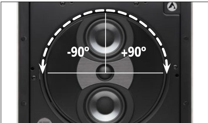
M-T-M baffle can be rotated 90 degrees from center. Do not exceed this rotation angle to avoid putting undue stress on the midrange-tweeter lead wires.
