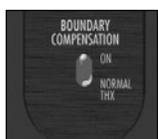
Large room boundaries, such as floors, walls, and ceilings, reinforce sound by acting essentially as acoustic “mirrors.” When the speaker is mounted too close to the corner or a wall/ceiling intersection, this sonic “reinforcement” often results in an unnatural heaviness or coloration of the sound.
