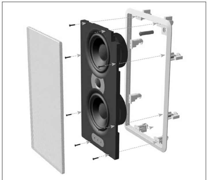
Once the frame is mounted in the wall, the speaker simply fits into the frame. Note that there is a gasket around the edge of the MDF baffle. This gasket ensures an airtight fit between the baffle and the frame. Therefore, the baffle may fit tightly in the frame. This is normal.
