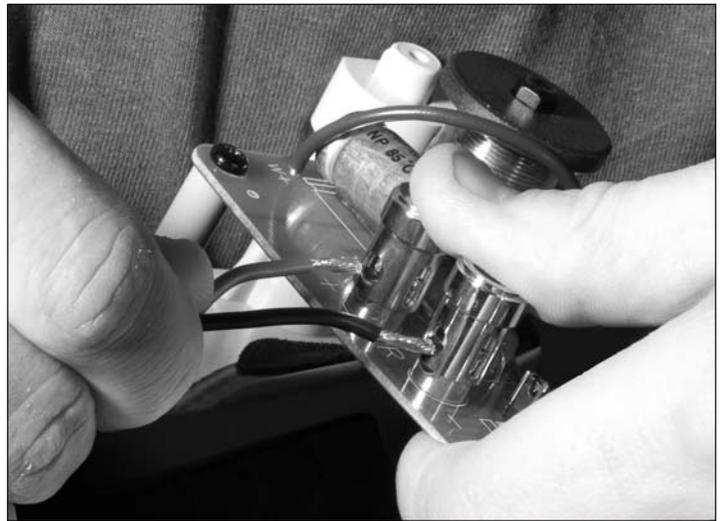
Strip about ½" (13 mm) of insulation from the connecting wires. Connect them to the appropriate push terminal, being careful to observe polarity (positive to the red terminal, negative to the black terminal).
