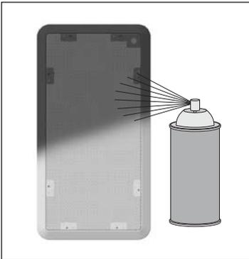
The white plastic frame and the metal grille may be left as is, or painted to match your décor. You can paint the frame before or after it is installed in the wall. Spray painting (using slightly thinned paint) is the best method to use for painting the grille. After painting the grille, use air pressure to "blow out" any grille holes that are filled in with paint.
